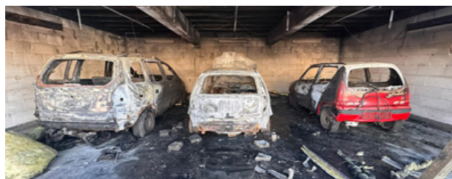
Test no 2 – i-Sprink kit deactivated (no fire suppression)
