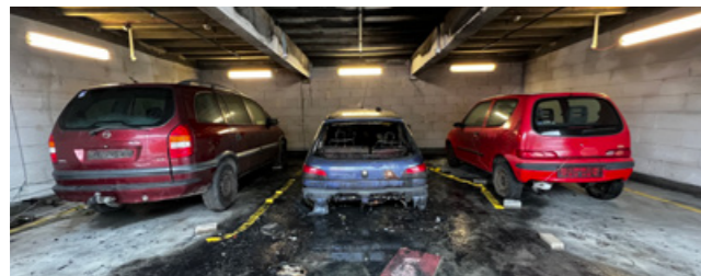
Test no 1 – i-Sprink kit activated (automatic fire suppression)
