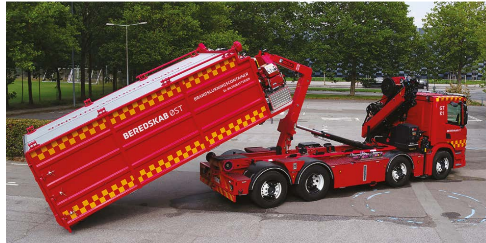
Dipping container intended for extinguishing electric and hybrid (li-ion) cars fires
