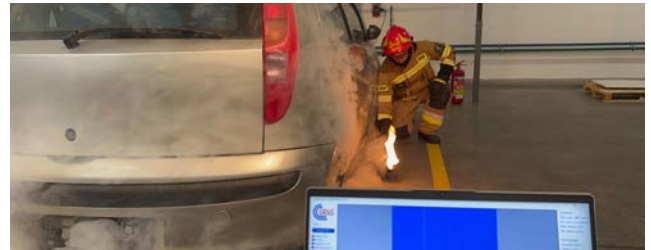
View of the test rig used for the real-scale assessment of the innovative fire risk detection and localization system
