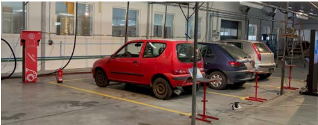
View of the test rig used for the real-scale assessment of the innovative fire risk detection and localization system
