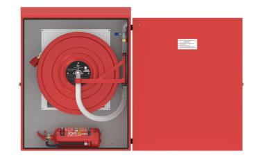
OUTDOOR HEATED AND INSULATED HYDRANT, FOR WALL-MOUNTED WITH PLACE FOR AN EXTINGUISHER For outdoor use in cold conditions up to -25°. Thermostatically controlled heating unit and insulation secure cabinet interior against cold.
